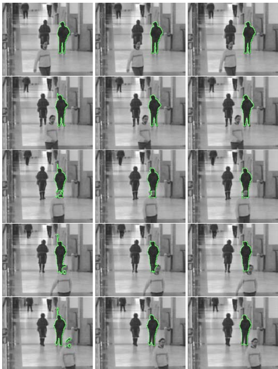
Fig. 3. Segmentation of a person covered by an occlusion in the human walking sequence. Left Column: without interaction term, Middle Column: \gamma = 20 , and Right Column: \gamma = 70 .
