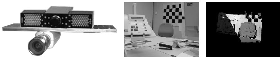
Fig. 1. 2D/3D-camera rig with image pair, PMD-image mapped to match 2D-image
