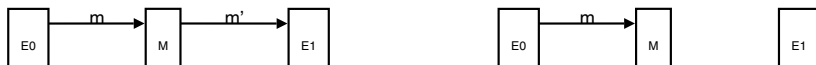
Fig. 3. A message m from endpoint E_0 to endpoint E_1 is forwarded (left) or dropped (right) by the midpoint M
