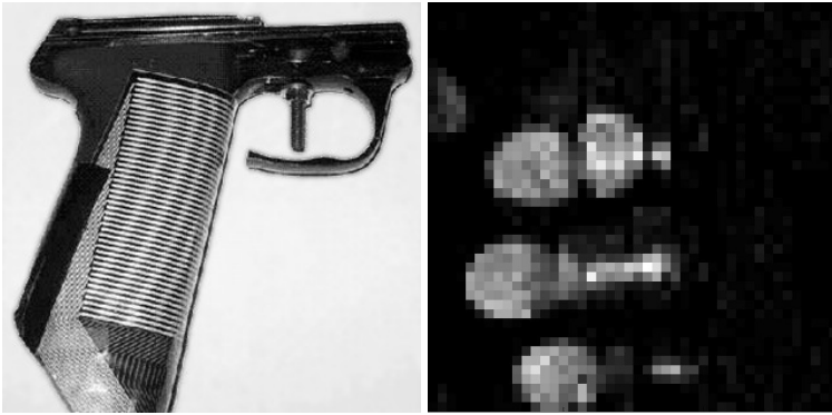
Fig. 1. Left: prototype of the smart gun. Right: an example of grip-pattern image.
