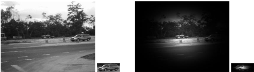
Fig. 1. Blackman window modulation distorts images. ( left ) Original search image and template; ( right ) Modulated search image and template.
