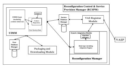
Fig. 2. Internal RCSPM architecture (not complete; only adaptability-relevant modules are depicted).
