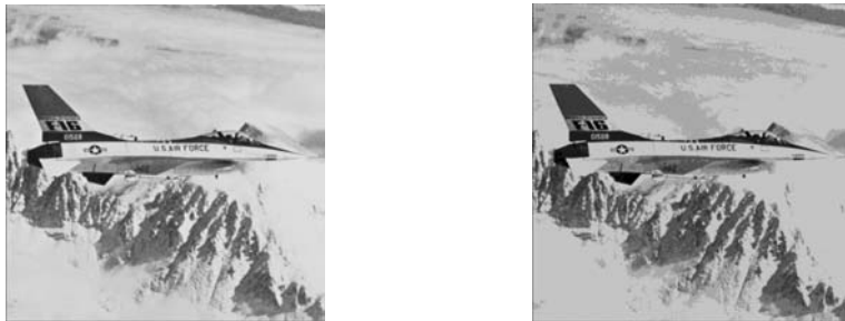
Fig. 2. Original image (left) and image coded with 9 gray levels (right)
