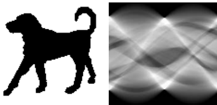
Fig. 2. A 2D shape and its Radon transform.
