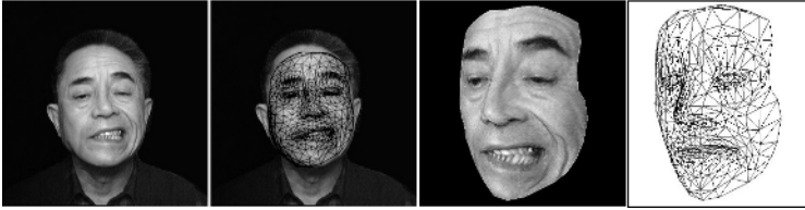
Fig. 3. The altered mesh of the grin expression and 3D models generated by applying z-values of corresponding range data.
