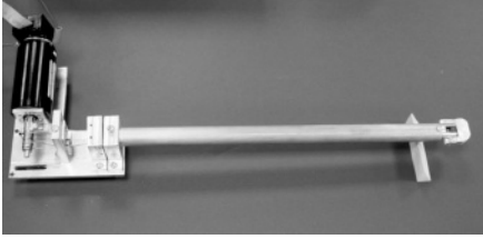
Fig. 2. Prototype of the laparoscopic grasper with force feedback.
