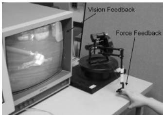
Fig. 4. Subject interaction with PHANToM to obtain force feedback from the grasper.
