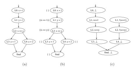
**Fig. 1.** (a) The CFA for our example program, (b) The CFA labeled with inferred predicates if  $\mathcal{P} = \{(x == y)\}$ , i.e., it contains the only branch in the program, and (c) The abstract automaton  $\mathcal{A}(\Pi, \mathcal{P})$ , which proves that L4 is not reachable.
