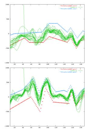
Fig. 3. Gyroscope Readings in the lateral and saggital plane over 10 Steps. Linear Approximation of the Safe Zone
