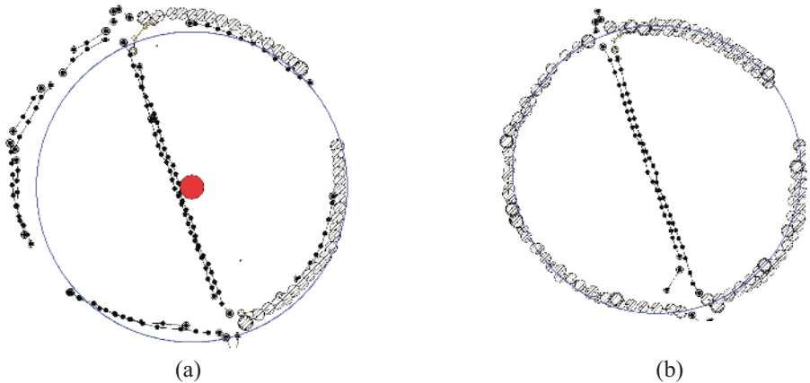
Fig. 5. The position and radius of the initial circle is refined. Points which are considered to originate from the circle are shaded. Initially (a), only the points of curved point sequences are considered to be part of the circle. Thus, the initial circle is not optimal. In (b) additional points have been determined by identifying point sequences which are close to the initial circle. The initial circle is iteratively adjusted to the points by Landau's method [12]. Only few iterations are required (two iterations in this example)
