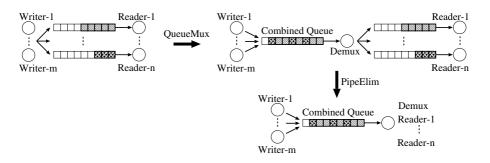
Fig. 5. Applying the QueueMux Transformation, followed by PipeElim
