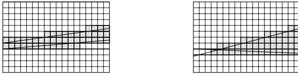
Fig. 4. Discrete epipolar line obtained from epipolar inequalities: two examples without (left) and with (right) an epipole
