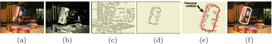
Fig. 7. Steps to extract the exact position of the object fusing color segmentation and accurate adjustment by deformable contours (commented in the text).
