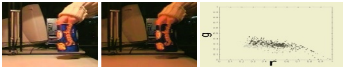
Fig. 1. Example frames of a sequence with time-varying color illuminant and its corresponding color distributions (in normalized rg color space).
