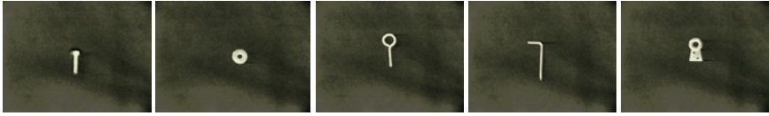
Fig. 1. The five objects used in the experiments. (a) A bolt. (b) A washer. (c) An eyebolt. (d) A hook. (e) A dovetail.
