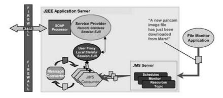
Fig. 8. CIP file notification process
