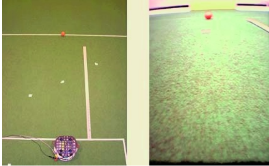
Fig. 6. Placement of the ball and test locations relative to the robot, as seen from (a) an overhead view and (b) the robot camera
