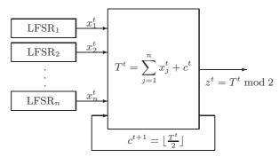
Fig. 1. Structure of summation generators
