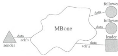
Fig. 1. Main elements present in a VLMCC transmission.
