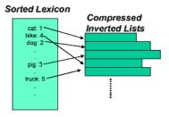
Fig. 3. Inverted file produced by the Flusher.
