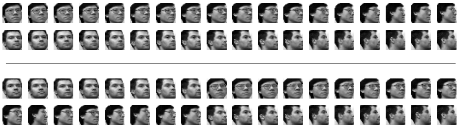
Fig. 6. Two-dimensional manifold discovered by TIE. Top two rows show first dimension, bottom two rows show second dimension. Note: first dimension captures rotation, whereas second captures frontal views versus side views.
