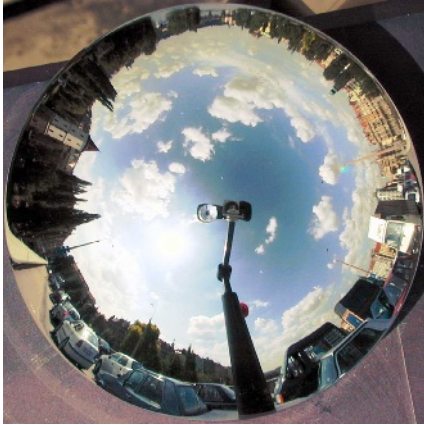
Fig. 1. An omnidirectional image obtained using a hyperbolic mirror and an ordinary perspective camera. Note the typical predominance of the sky.
