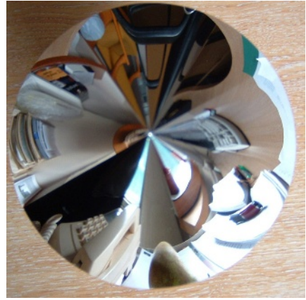
Fig. 2. A conical mirror image of an indoors scene. The entire mirror image reflects useful data.
