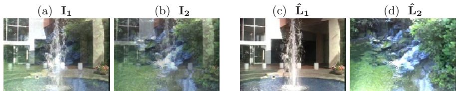
Fig. 3. Handling spatially varying mixing functions. (a)-(b) The two mixtures I_1 and I_2 were obtained by mixing two images ("fountain" and "waterfall") with 4 different non-linear functions ( \alpha_1 was a sinus, \alpha_2 and \beta_1 were two exponent functions, and \beta_2 was a constant function). (c)-(d) The recovered transparent layers using our global-to-local layer separation method described in Section 3.2 .
