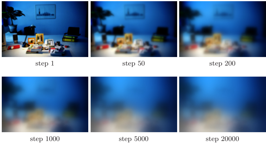
Fig. 3. Local space average color is computed iteratively. The images show local space average color after 1, 50, 200, 1000, 5000, and 20000 steps. For this image 22893 steps were needed until convergence.
