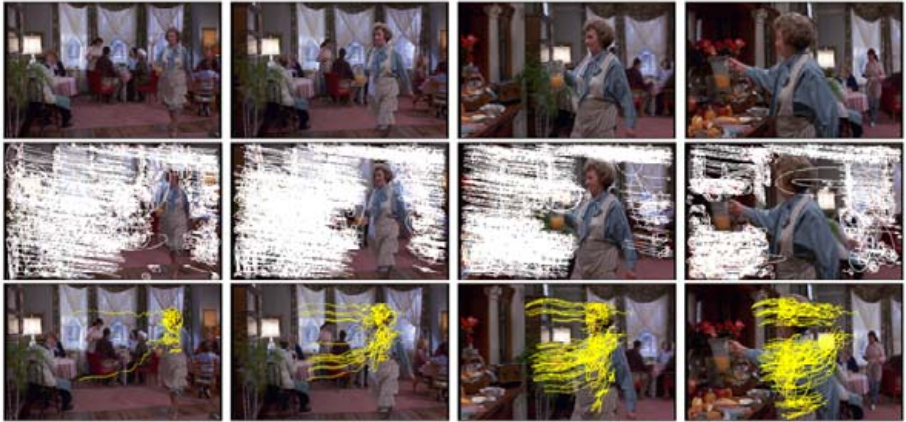
Fig. 7. Example III: object level grouping for another (83 frame) shot from the movie Groundhog Day. Top row: The original frames of the shot. Middle and bottom row: The two dominant (measured by the number of tracks) objects detected in the shot. The number of tracks associated with each object is 225 (landlady) and 2764 (background). The landlady is an example of a slowly deforming object.
