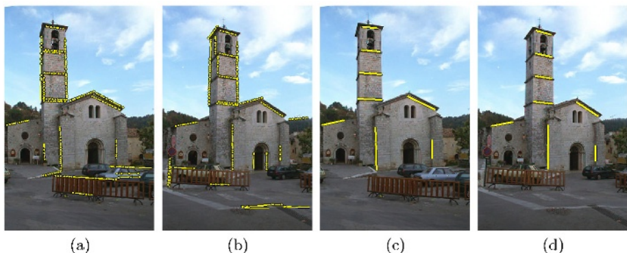
Fig. 1. (a) & (b) Show the detected POPs. The repeatability rate is 51% while for points and lines it is lower, respectively 41% and 37%. (c) & (d) show the 9 putative matches obtained with our algorithm. On this example, all of them are correct, which shows the robustness of our local geometry based cross-correlation measure.
