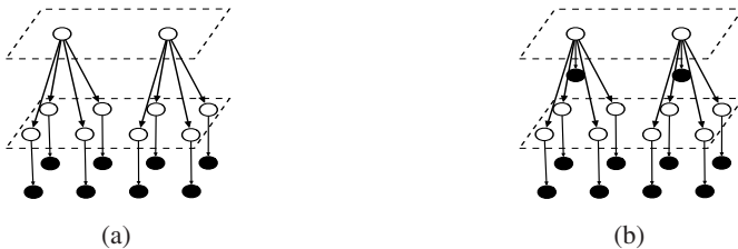
Fig. 1. Differences in TSBN models: (a) observable variables at the lowest layer only; (b) our approach: observable variables at all layers. Black nodes denote observable variables and white nodes represent hidden random variables connected in a tree structure.
