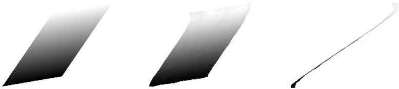
Fig. 4. Left: true depth map of the scene. Middle: recovered depth map. Right: profile of the recovered depth map. As can be noticed, the recovered depth map is very close to the true depth map with the exception of the top and bottom sides. This is due to the higher blurring that the images are subject to at these locations.
