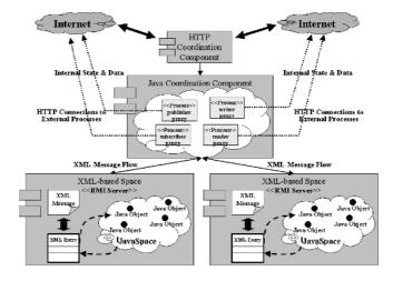
Fig. 2. Software Components of the coordination service
