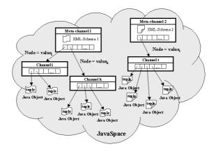
Fig. 5. Partition based on meta-channels and channels
