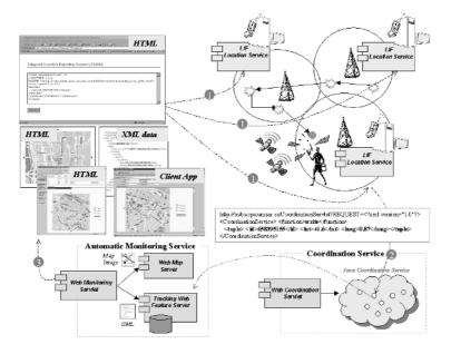
Fig. 8. Deployment architecture for tracking delivery parcels.
