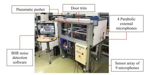
Fig. 1. The in-process BSR noise detection system.
