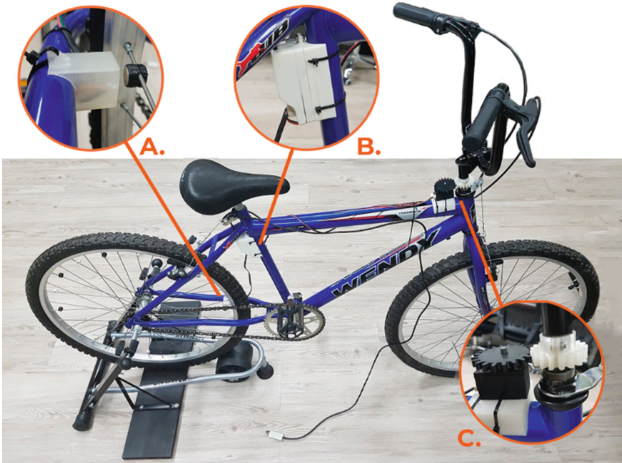
Fig. 1. Bicycle system with the sensors. A: Hall sensor and magnets. B: Arduino board attached to a case. C: Potentiometer and 3d printed gears
