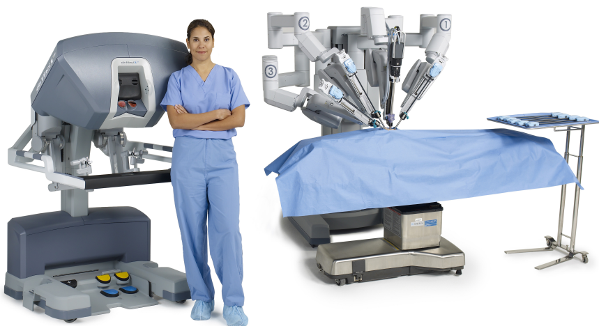
Figure 4.3: The da Vinci assistance system (©2014 Intuitive Surgical, Inc) with the workstation on the left and the distant robotic system on the right.
