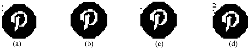
Fig. 7. Recovered watermarks after attacks by: (a) Compression JPEG_50, (b) Translation_20, (c) Gaussian noise_0.01, (d) Rotation_0.5°
