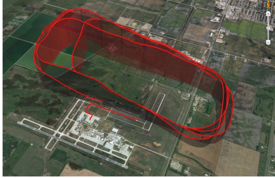
Fig. 1. Example of using a KML file to visualize a flight path in Google Earth. This flight visualization is an example of a student flight that has multiple final approach phases.
