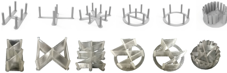
Fig. 4. Analysis process of the toolpaths (stringing) generated by Slicer software
