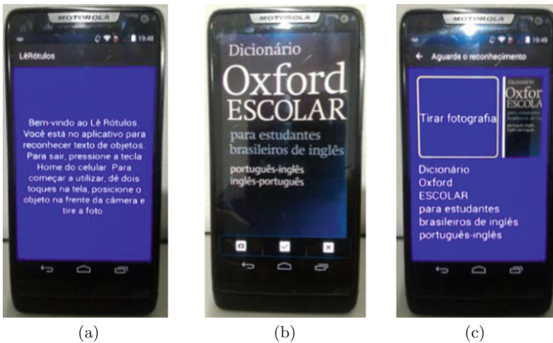
Fig. 1. LêRótulos screens. (a) Initial screen with instructions for use. (b) Photography of an object. (c) Recognized photo data.
