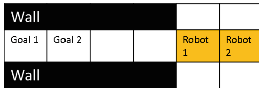
Fig. 7. Hallway example where the total cost (Euclidean Distance) for Robot 1 to Goal 2 and Robot 2 to Goal 1 is identical to the Robot 1 to Goal 1 and Robot 2 to Goal 2. It is arbitrary which goal the Hungarian Algorithm will assign with a Euclidian distance cost function, leading to cases when robots are blocked.
