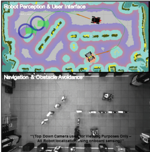
Fig. 10. Hardware demonstration of user interface and robot control. Two robots are autonomously navigating to the assigned goals.
