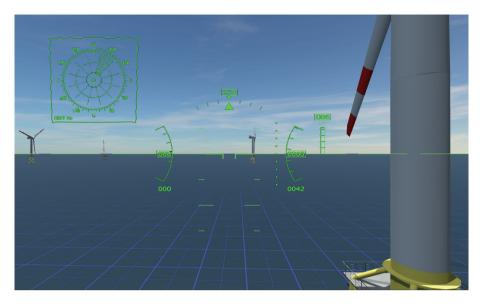
Fig. 9. HWD OAWS in case of conducting a hoist operation at the lower access point of an offshore wind turbine
