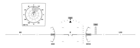
**Fig. 7.** Orthogonal coplanar 360 degree top view in a HWD depicting surrounding obstacles (Color figure online)
