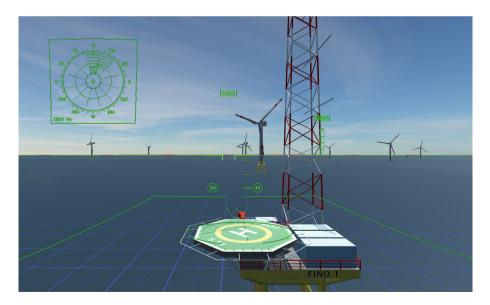
Fig. 10. HWD OAWS in case of landing on the research offshore platform FINO1
