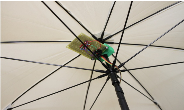
Fig. 2. Sensor part of ii-kasa
