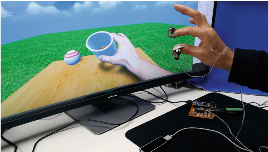
Fig. 1. A 3D virtual reality system that uses pseudo-force perception produced by DC motor rotational acceleration to present stiffness feedback sensations to the tips of the thumb and index finger during grasping of a virtual tube. We modulated the visual feedback by changing the cross-sectional shape of the tube from a circle to an ellipse.
