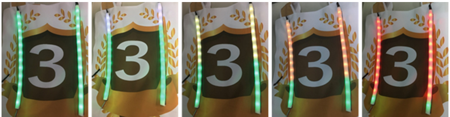
Fig. 7. Relationship between color and life points (Left: all green indicates maximum life points, Right: most of LEDs turns red to indicate exhausted life points) (Color figure online)
