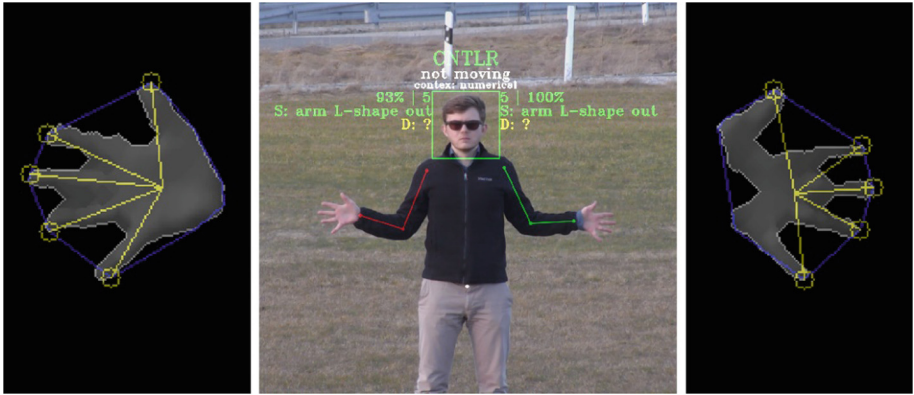
Fig. 6. Visualization of the onboard gesture recognition and finger detection algorithm, from top to bottom line: 1. CNTLR = Count fingers on left and right side, 2. movement status, 3. current context, 4. Number of detected fingers and confidence for each hand, 5. S = detected observation of static gesture recognition, D = result of dynamic gesture recognition (here none, since operator is not moving), yellow circles = detected finger tips (Color figure online)
