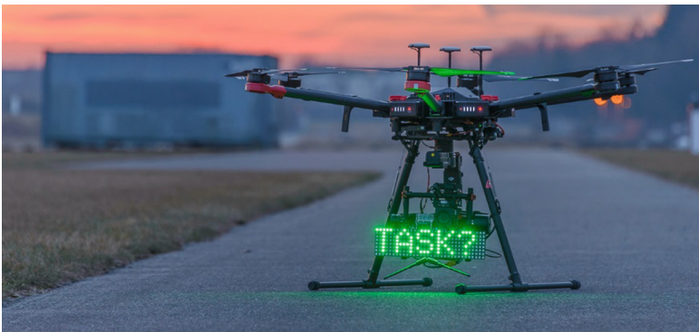
Fig. 7. Multicopter UAV with stabilized sensor system, processing board and LED matrix for visual feedback
