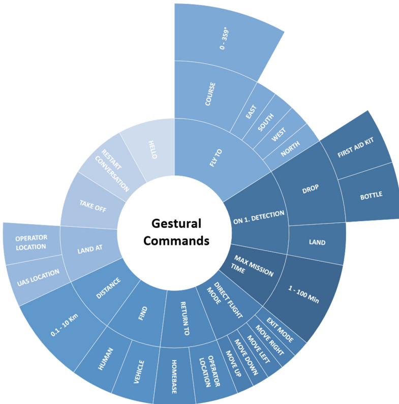
Fig. 5. Supported gestural tasking commands and the task dependent additional information
