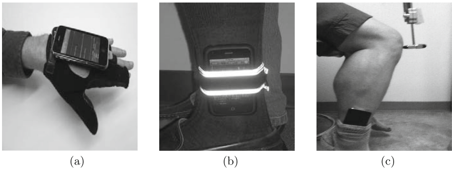
Fig. 11. Secure iphone to hand or ankle: (a) Glove; (b) Elastic bands; (c) Socks.
