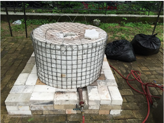
Fig. 4. A simple outdoor raku kiln
