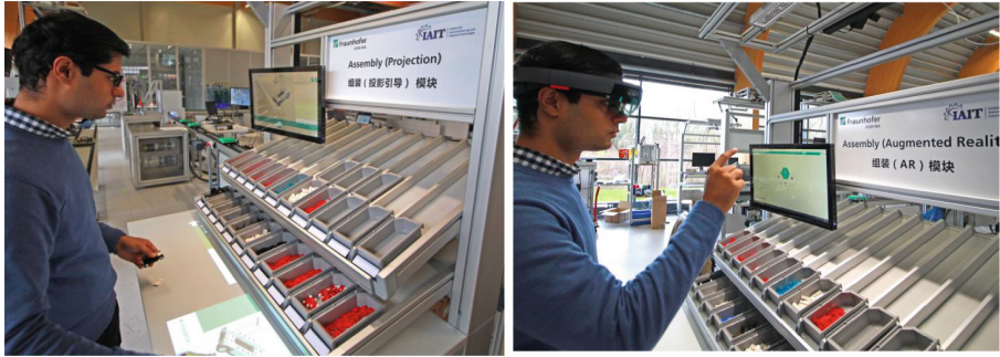
Fig. 3. System setup with projection-based display (left) and HoloLens (right).
