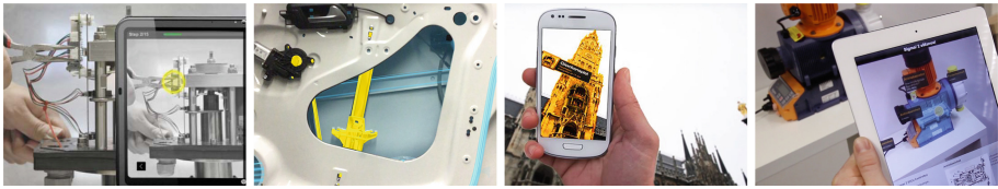
Fig. 2. Range of highlighting elements (left to right): (a) semi-transparent, circular indicator enclosing the point-of-interest, (b+c) shape and geometry-based yellow highlight make target objects protrude [22], (d) highlight as selection indicator: similar to the prior, the object's contour is used as highlight boundary, here interactively triggered at the target object through a gaze-technique. (Color figure online)
