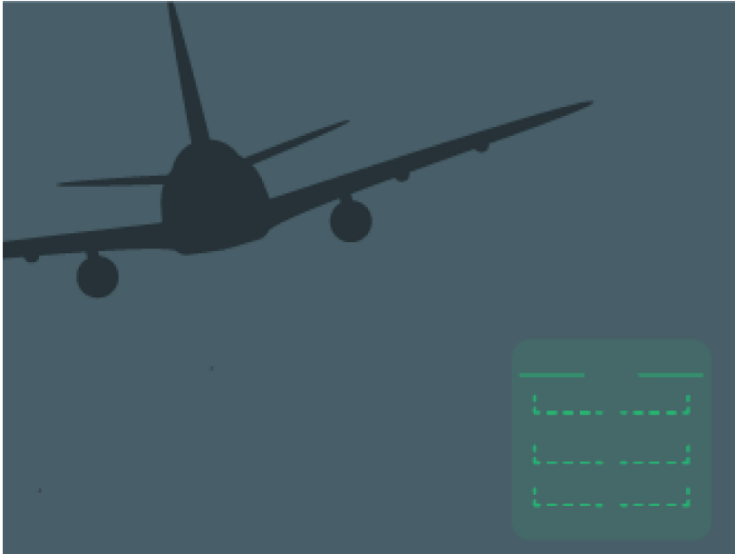
Fig. 2. Extended off-axis pitch ladder design. The pilot is looking off-axis, up and to the left. This design extends the traditional pitch ladder by removing aircraft/route indicators, changing the location/size of the pitch ladder by reducing the size and placing it in the lower right corner, and employing a background for additional cueing that this pitch ladder represents on-axis information.
