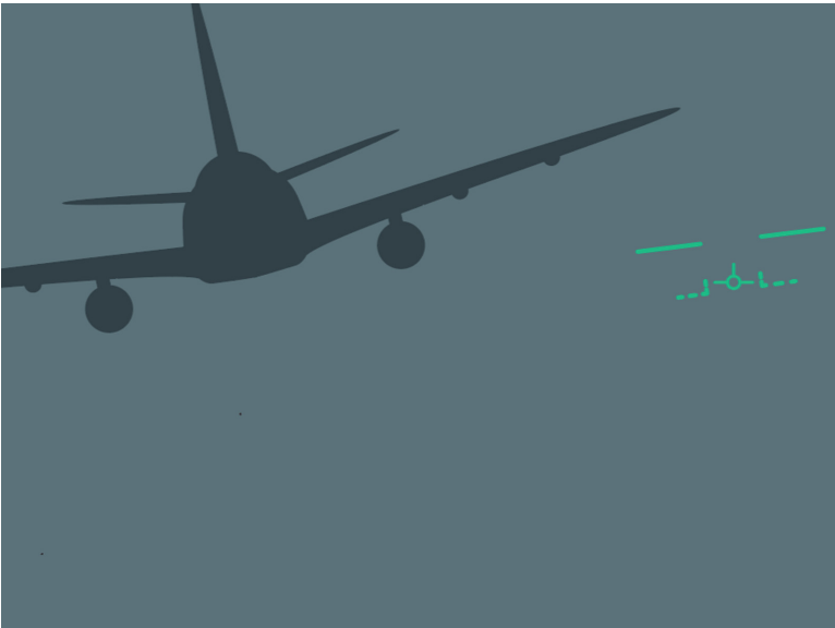
Fig. 5. “Minimal” extension to traditional pitch ladders for off-axis context indicating a slight pitch down and slight roll
