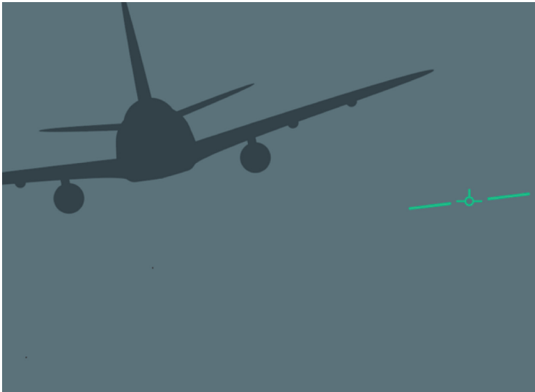
Fig. 3. “Minimal” extension to traditional pitch ladders for off-axis context indicating a slight roll
