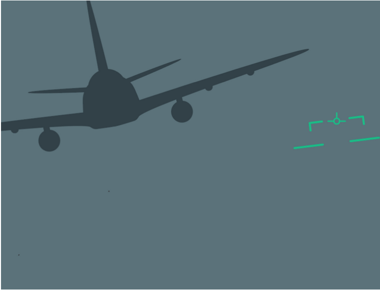
Fig. 4. “Minimal” extension to traditional pitch ladders for off-axis context indicating a slight pitch up and slight roll
