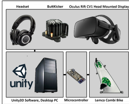
Fig. 4. Schematic of the VR setup
