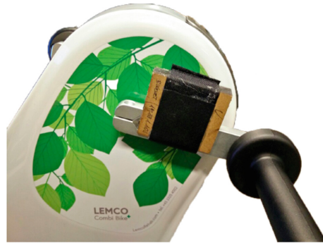
Fig. 3. The GIRO microcontroller [14] strapped to the pedal arm of the Combi Bike
